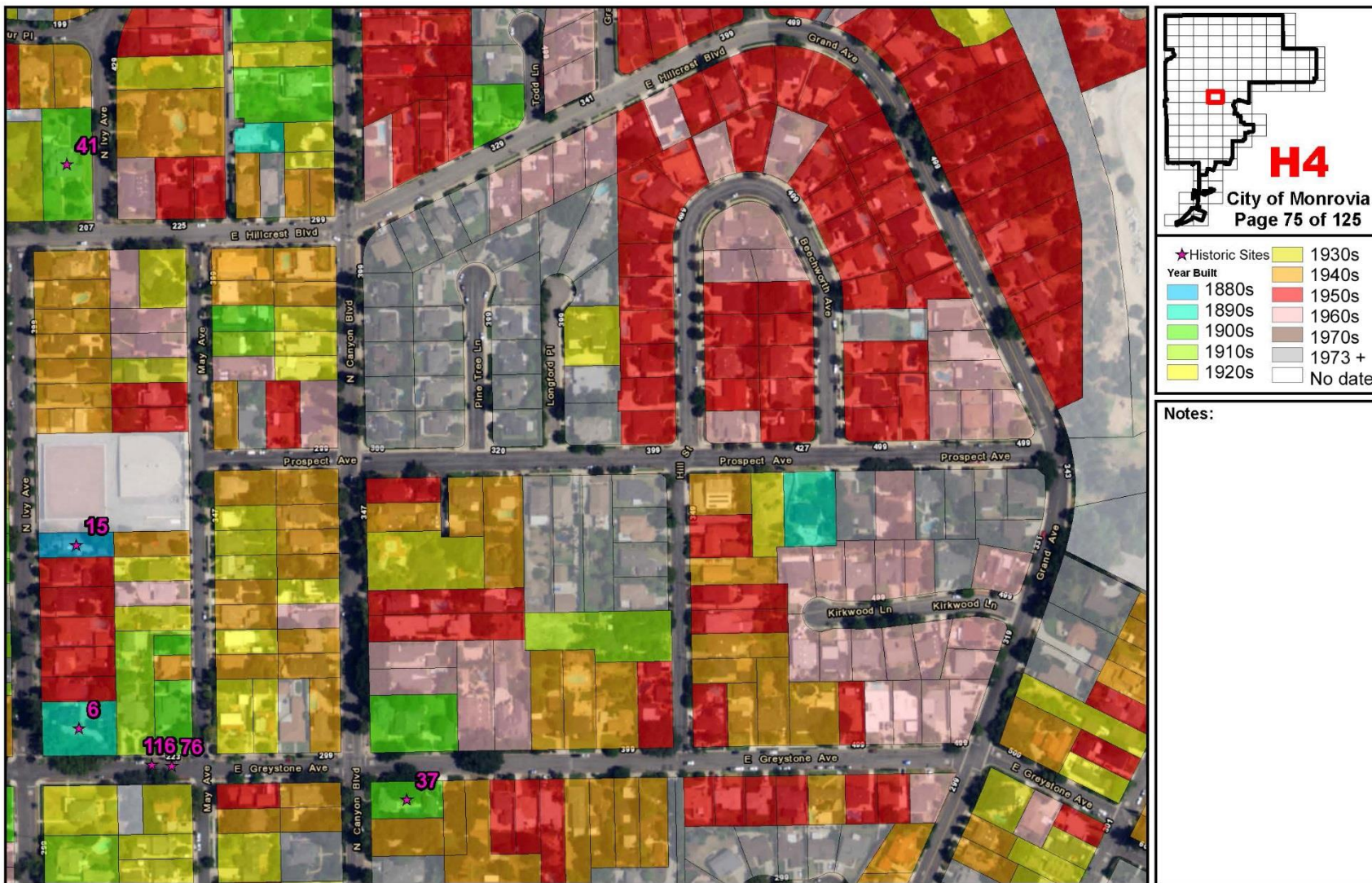
Figure 2.3 Example of reconnaissance survey map, with parcels identified by decade of construction.
