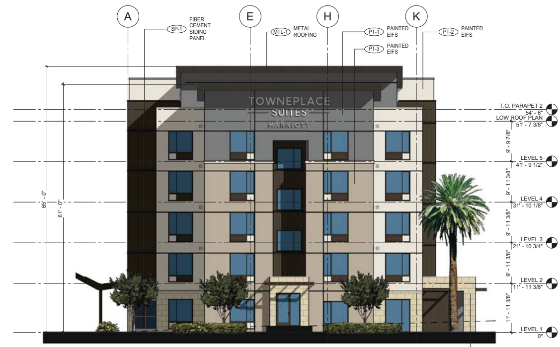
EXTERIOR EAST ELEVATION
