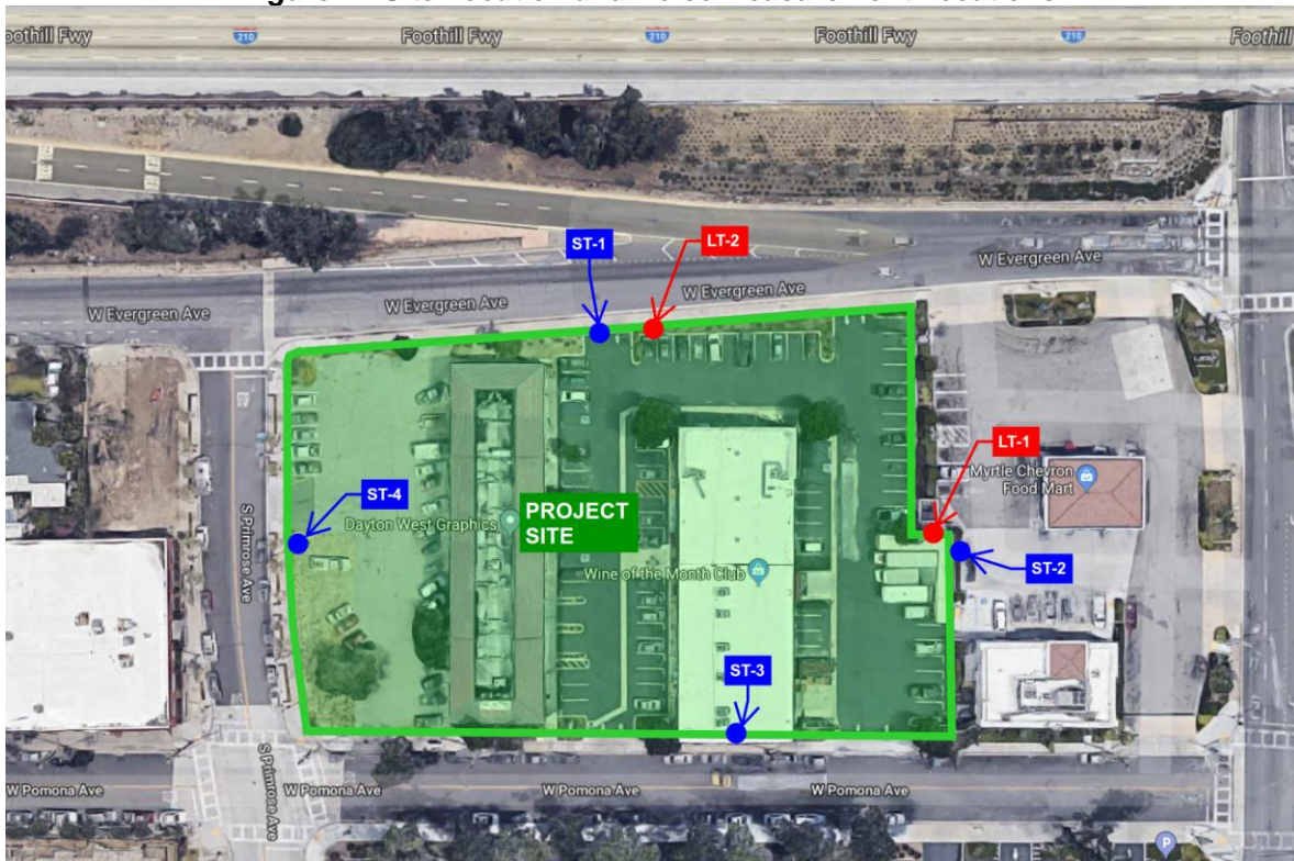
Figure 2: Site Location and Noise Measurement Locations
