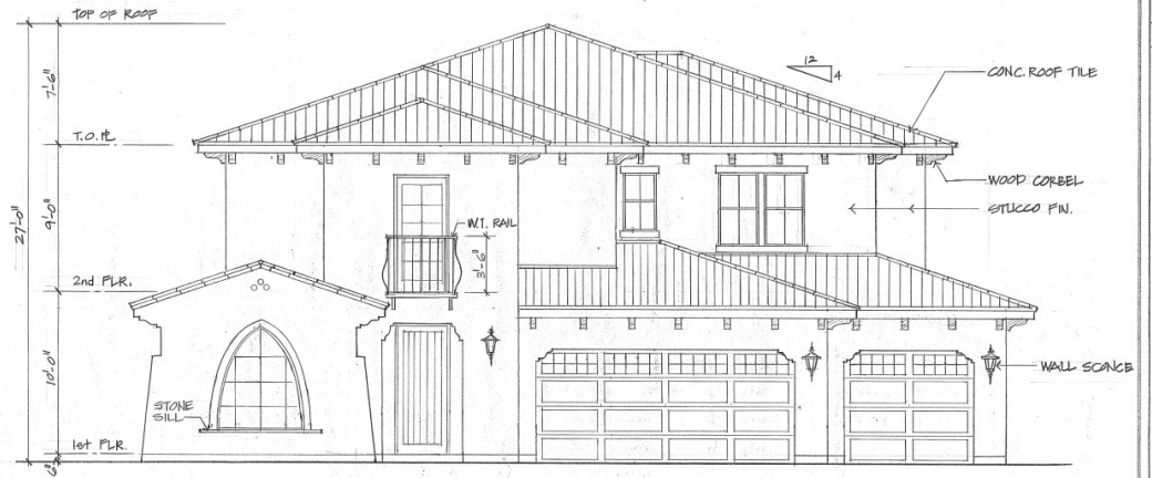
UNIT A EAST ELEVATION \frac{1}{4}'' = 1'-0''
