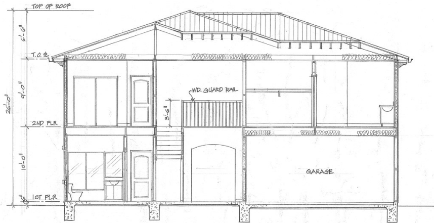
UNIT "B" SECTION "B-B" \frac{1}{4}'' = 1'-0''
