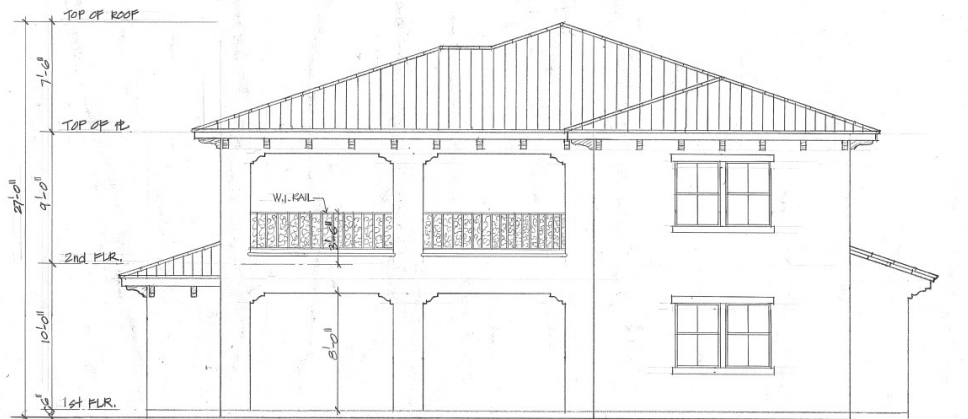
UNIT A WEST ELEVATION \frac{1}{4}'' = 1'-0''
