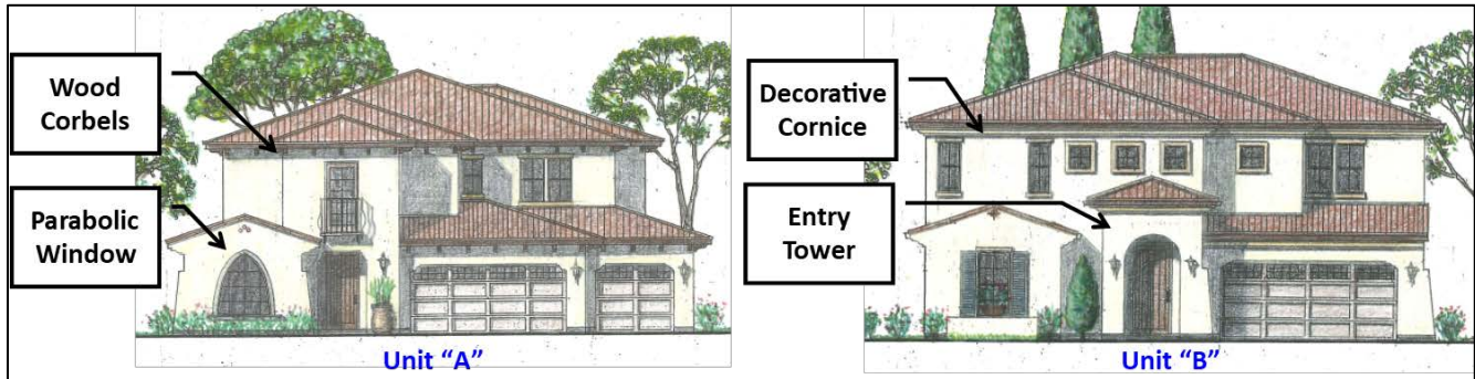
Figure 3. Front Facades of Units A and B
