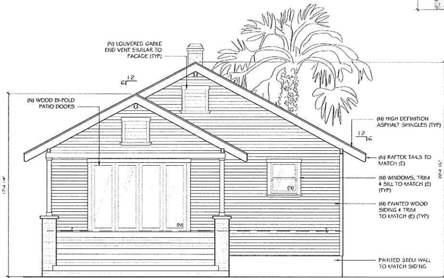
SOUTH ELEVATION (AREA OF ADDITION) SCALE: 1/2" = 1'-0"
