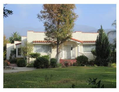
(south) elevation. Round Doric posts support the front-gabled porch roof. Concrete steps lead to the front entrance (obscured by a non-original metal security door) and a pair of flanking sidelights. Wide fixed picture windows shaded by red-tiled shed roofs are located east and west of the entrance. An exterior red brick chimney rises from the east elevation. The single-family residence is of wood frame construction and rests on a raised foundation.
