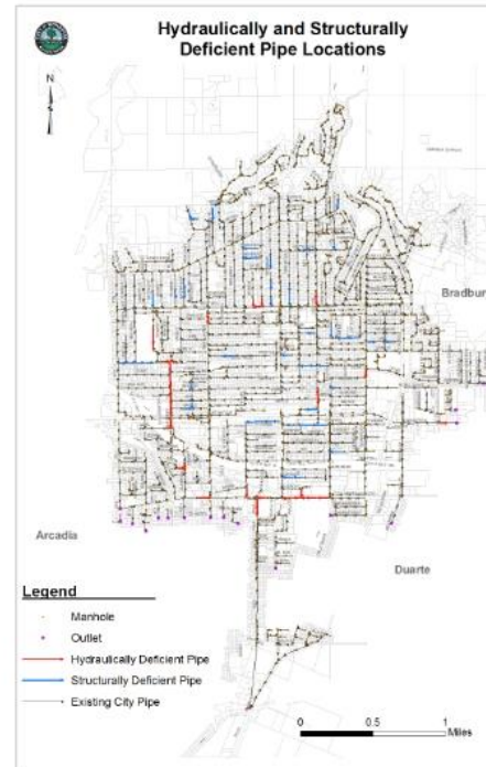
Figure 7-1 Hydraulically and Structurally Deficient Line Segments
