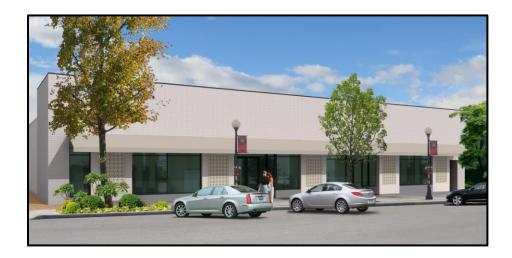
The façade remodel proposes to retain the original brick building's midcentury aesthetic as much as possible. All design elements that were added for decoration in the 1980s will be removed, including the green cornice trims at the top of the building, the green light fixture that spans the entire length of the storefront, and the ceramic red tiling.
